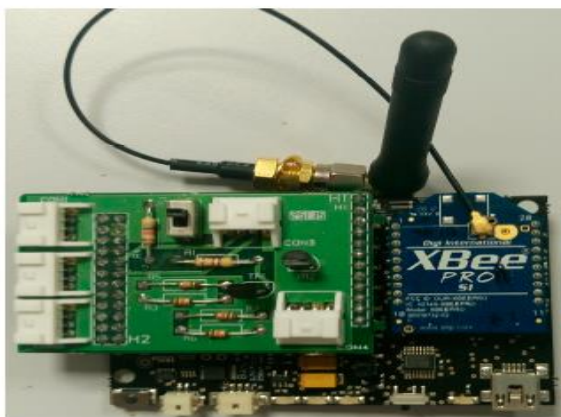
Figure 3. UcoBee Version 1 wireless node.
