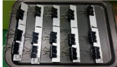
Fig. 3 Single-lap-joint adhesively bounded sample are ready put on the oven for curing process
