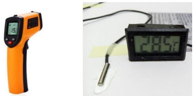
Fig. 5 Non-contact infrared temperature gun (L) and Thermocouple (R)
