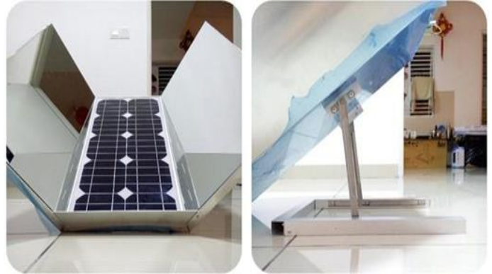
Fig. 3 Front (L) and side view (R) of the 60^\circ VTC with PV Panel [2]
