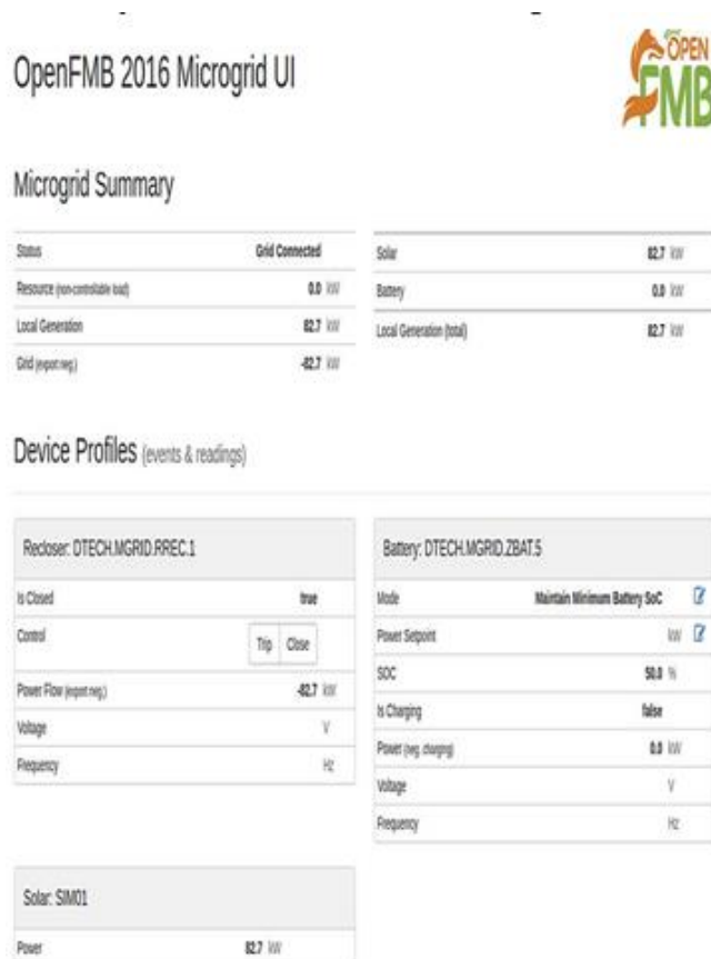
Fig. 4 Visualization of Microgrid using OpenFMB framework
