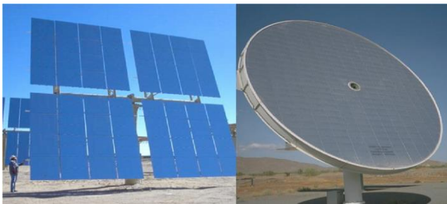
Fig. 2 Heliostat geometry types: (A) Lugo, tested in Solar-Two plant, (B) stretched membrane, tested in, Spain [19]
