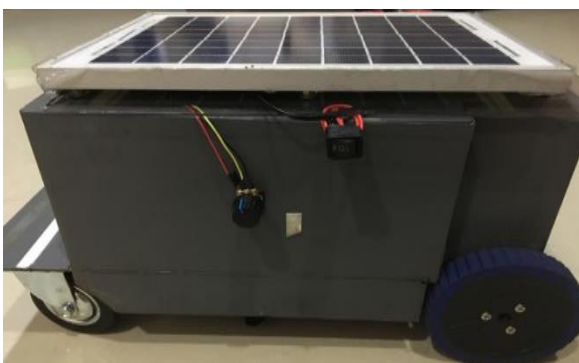
Fig. 6 Prototype of smart solar grass cutter
