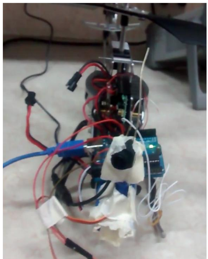
Fig 5. Camera mounted on servo motor
