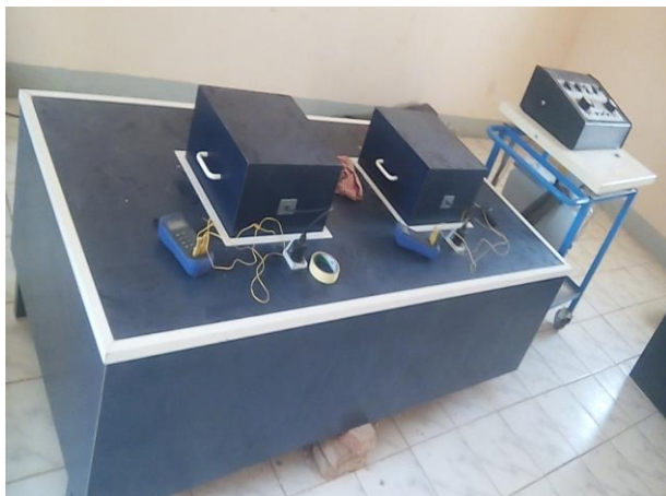
Fig. 3. Measuring device for thermal conductivity EI 700
