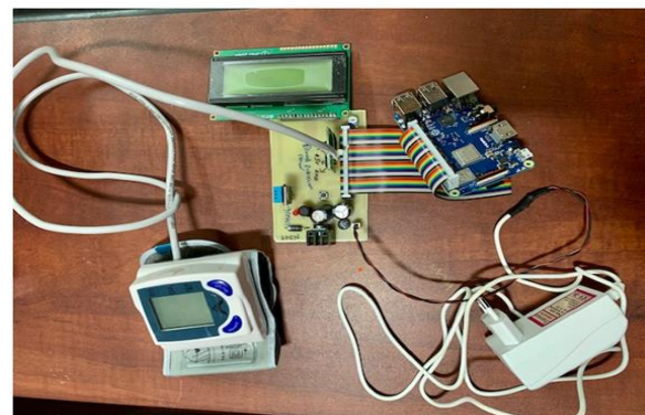
Figure 2: Hardware set-up for proposed tele-healthcare unit
