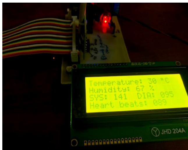
Figure 4: patient systolic, diastolic and heart beat rate on proposed tele healthcare Unit
