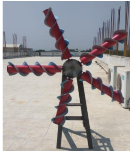
Fig. 5. Horizontal axis Magnus wind turbine at testing
