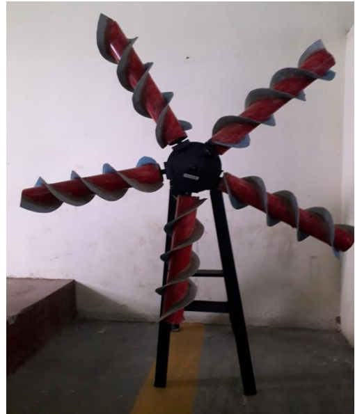
Fig. 4. Assembled horizontal axis Magnus wind turbine
