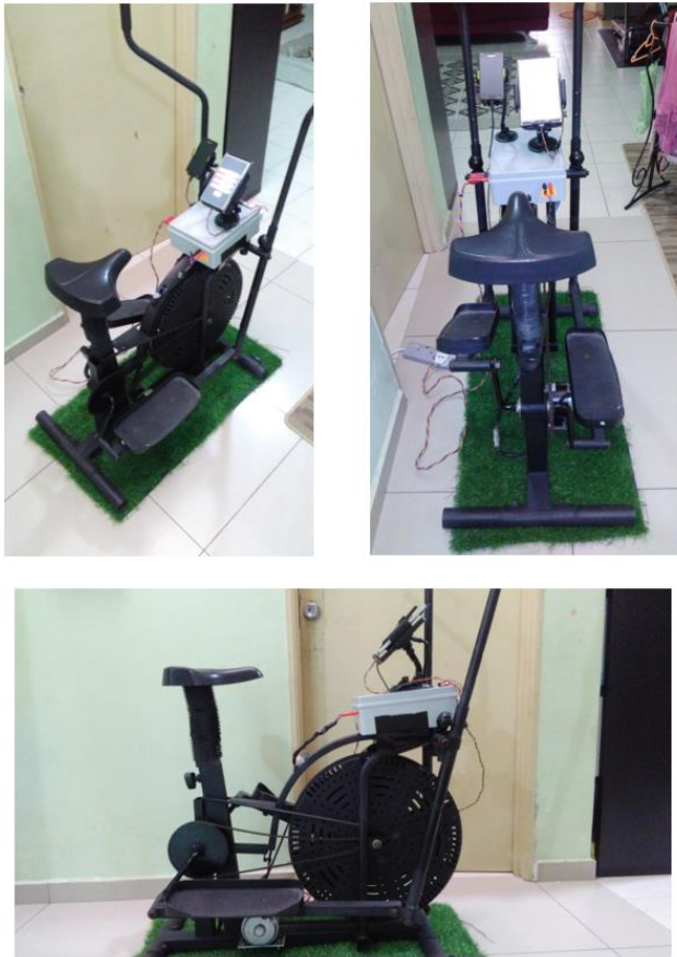
Fig. 10. The developed stationary cycling charger prototype.
