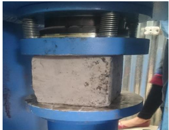
Figure 5 – Compressive Test of Cubes using CTM
