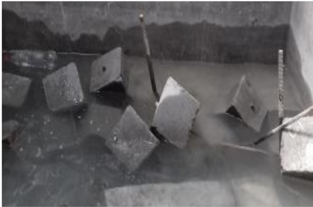
Figure 3 – Curing of Concrete Samples
