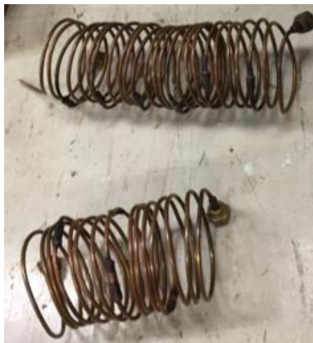
Fig. 5. Spiral coil of capillary tube
