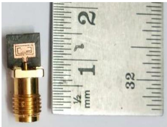
Figure 6. Fabricated prototype of the proposed antenna
