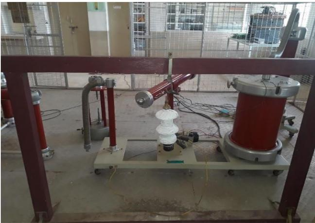
Fig. 1. Tentative setup for pollution testing
