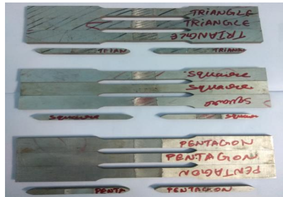
Fig. 9 Tensile specimens extracted from FSW weldments
