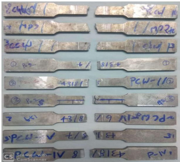
Fig. 12 GTAW tensile specimens after performing tensile test on UTM machine
