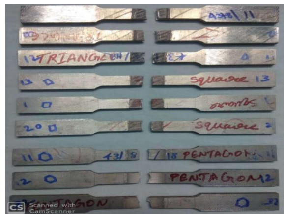
Fig. 10 FSW tensile specimens after performing tensile test on UTM machine
