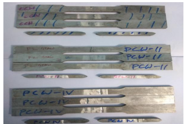
Fig 11. Tensile specimens extracted from GTAW weldments
