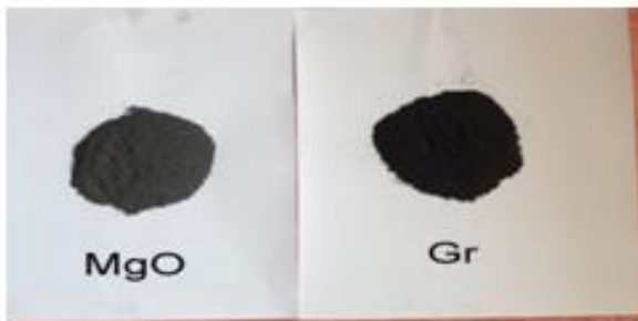
Figure 8: Reinforcement of sample
