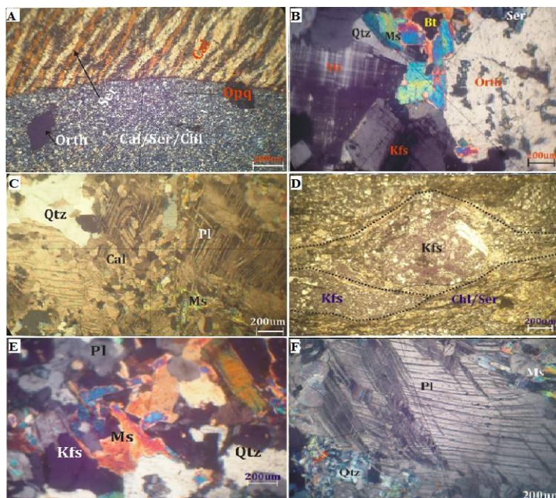
**Fig.2. Photomicrographs, A) sericite-chlorite schist under PPL, B) felsic volcanic rock under PPL; C) quartz-sericite schist under PPL; D) feldspar-sericite-chlorite schist under XPL (k-feldspars show sense of shearing due to deformation); E&F) plagioclase-muscovite-quartz rock under PPL (NB:Kfs-k-feldspar, Pl-plagioclase, Qtz-quartz, Chl-chlorite, Ms-muscovite, Ser-sericite, Cal-calcite, Mi-microcline, Bt-biotite,Orth-orthoclase, Opa-opaque).**
