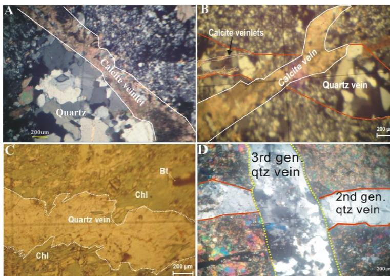
**Fig.3. Photomicrographs, A&B) Quartz-sericite schist cutting by quartz and calcite veins/veinlets under XPL, B) Chlorite-sericite schist cutting by second and third generation quartz veins under XPL (NB: Chl-chlorite and Bt-biotite).**
