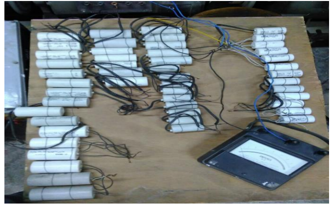
Fig. 4 Photo of the laboratory set-up of the capacitor bank used for IAG
