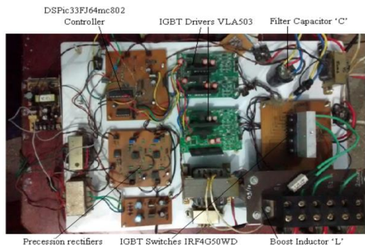
Fig. 19. Experimental Set-Up Of Laboratory Model
