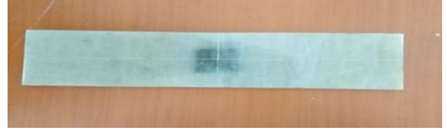
Fig. 5: With Delaminated Area of size 30\times 30\text{mm}^2
