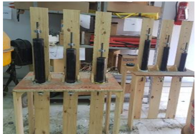
Fig. 7 install the bars to be spliced
