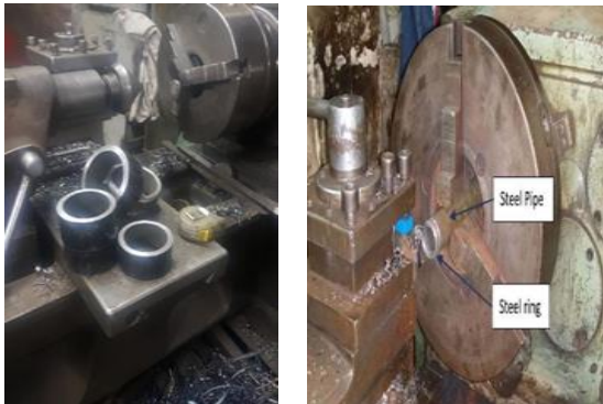
Fig. 6 Cutting the steel rings
