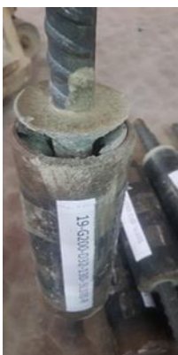
Fig. 9 Bar grout bond Failure
