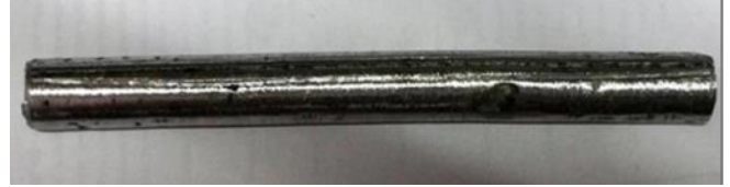
Fig. 11. Circular Specimen 15mm Diameter, 150mm length
