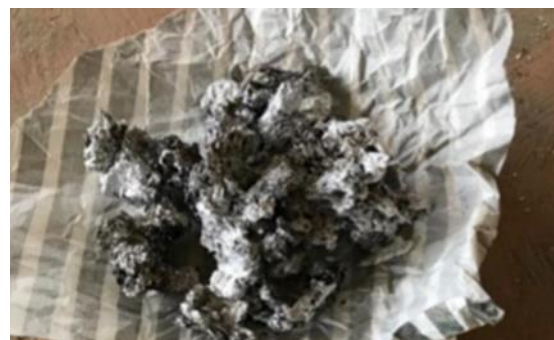
Fig. 13. Slag Collected after melting Plates and Panels
