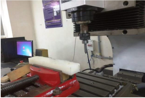
Figure 2 Experimental setup (high speed 3 axis vertical CNC machine)
