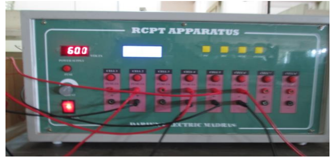
Fig. 2. Rapid Chloride Penetration test in progress
