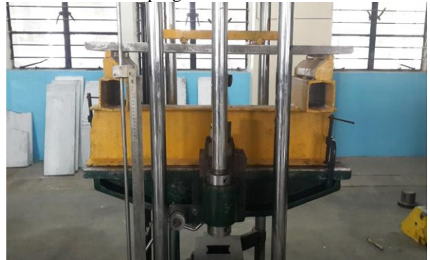
Fig.6 Flexural Strength Test Set up
