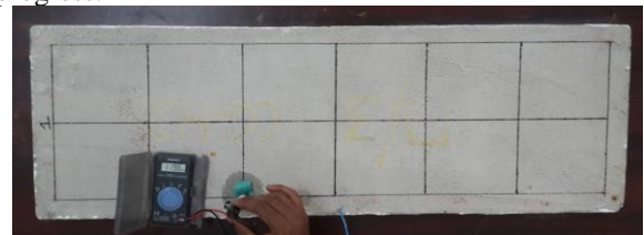
Fig.3 Half-Cell Potential test in progress
