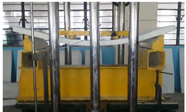
Fig.7 Flexural Strength Test in progress
