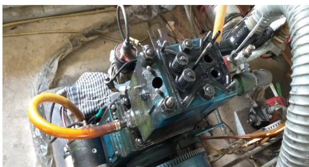
Figure 1: Variable Compression Ratio Kirloskar Engine.
