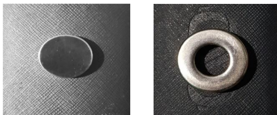
Fig. 6 Ring shape and Circular shape neodymium magnet
