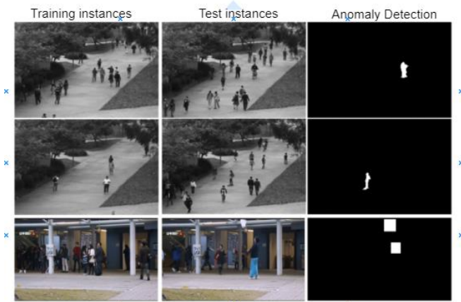
Fig 1. UCSD dataset ( top two rows) , portrays the appearance of a cyclist or a skate-boarder on the pavement as an unusual activity. In the Avenue dataset(bottom row), the throwing of papers into the air by a person accounts for an anomaly. The third row depicts the Avenue dataset wherein the propelling of an object in the air is identified as an anomalous event taking place. Since the person in the frame is throwing
