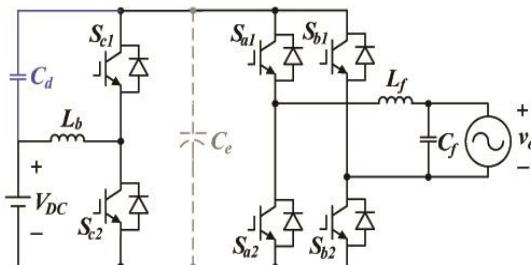
**Fig. 3. Bridge inverter built on buck-boost converter.**
