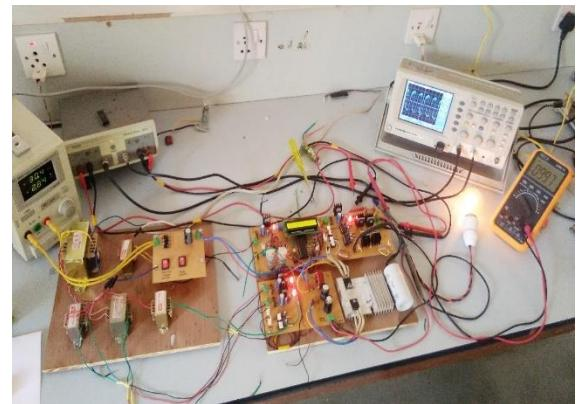
**Fig. 6. Hardware of the projected 1-φ bridge inverter.**
