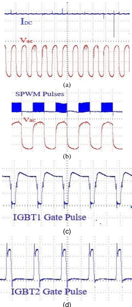
**Fig. 8. Experimental outcomes of the projected 1-φ bridge inverter: (a) Incoming DC current with output side AC Voltage (b) SPWM Pulses with respect to output voltage (c) Gate Pulse for IGBT1 of Buck-Boost converter (d) Gate Pulse for IGBT2 of Buck-Boost converter**
