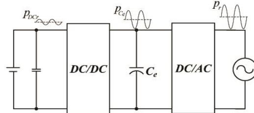
**Fig. 2. 2-stage 1- $\phi$  bridge inverter**
