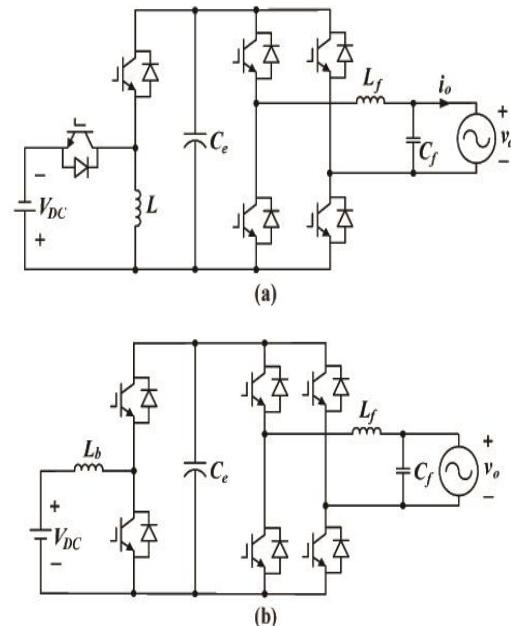
**Fig.1. 1- $\phi$  bridge type inverter with: (a) buck-boost convertor; (b) boost convertor.**
