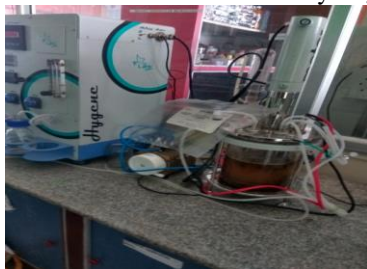
Fig 4.1 Anaerobic digester with Tedlar bag
