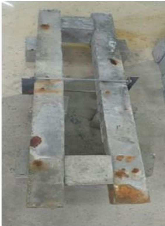
Fig. 6. Loading beams using steel frame connecting each two beams together
