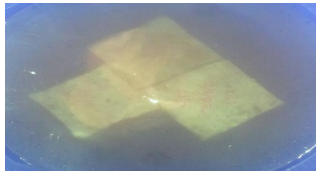
Figure.3 Cubes under curing in Sodium Sulphate solution
