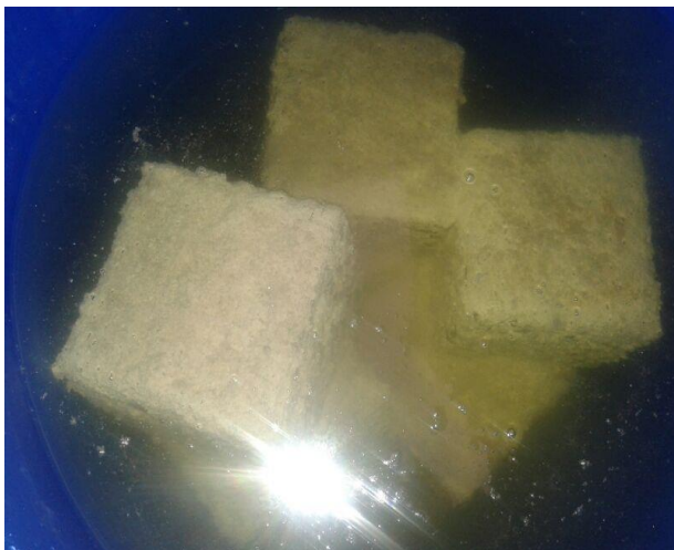
Figure. 5 Concrete cubes under curing in H 2 so 4
