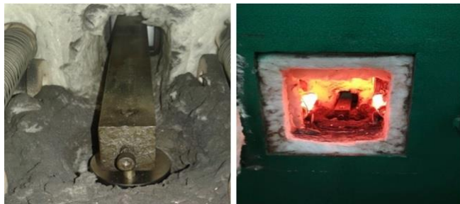
Fig.2 Pin and disc loaded condition in furnace
