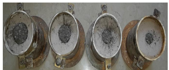
Fig.3. Installation of Stone columns of different diameters
