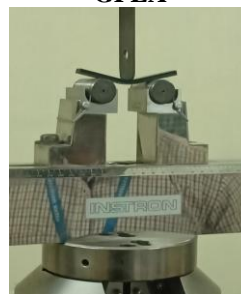
Figure 6(a). 3Point bending test - GLPA
