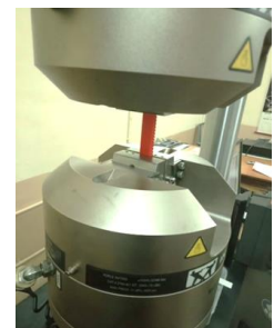
Figure 5(b). Tensile test on PTEG
