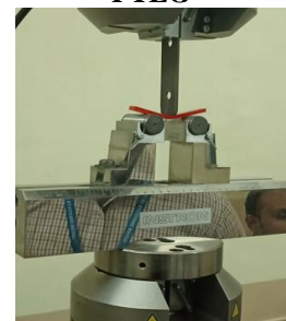
Figure 6(b). 3 Point bending test - PETG
