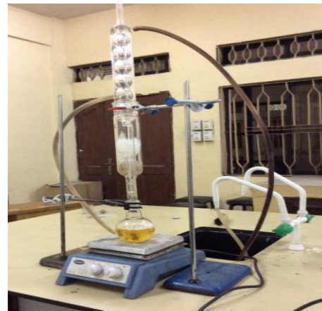
Fig. 2. Solvent Extraction Setup
