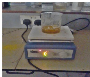
Fig. 3. Heating oil sample for solidification using stearic acid
