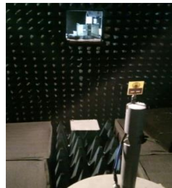
Fig.6. Proposed antenna in anechoic chamber.
