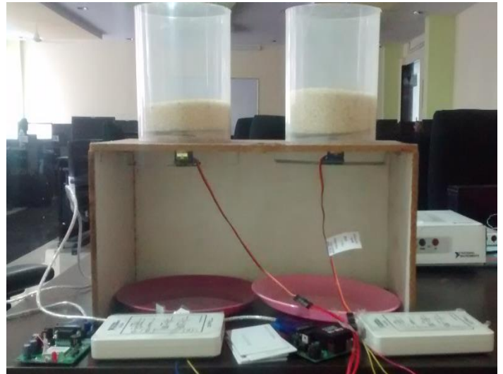
Fig 7: Prototype of Smart Ration Card System Using LabVIEW
