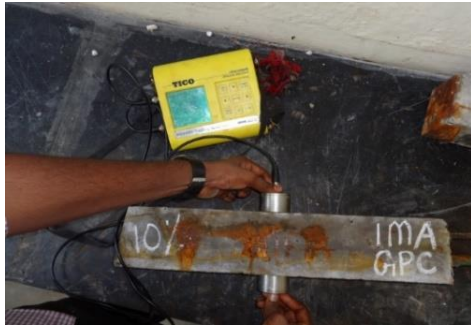
Figure 3.2: Testing of corroded specimens using UPV measuring Apparatus
