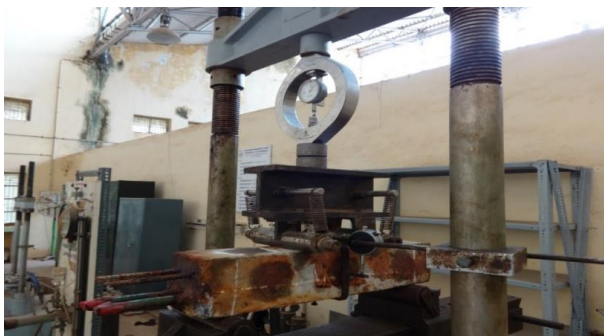
Fig.3.4: Arrangement for two-point bending test
