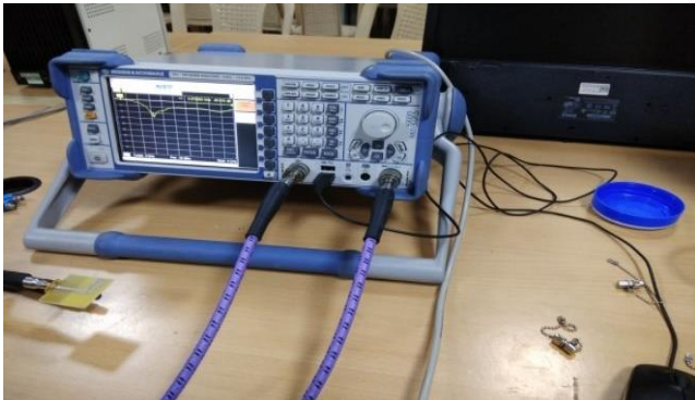
Fig. 11 Testing using Vector Network Analyzer
