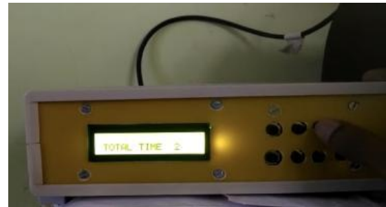
Fig.7 Selection of total time option for transferring the drug in the pump
