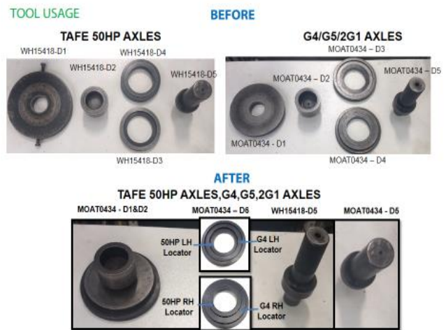
Fig. 4. Optimization of internal work by using proper fixture
