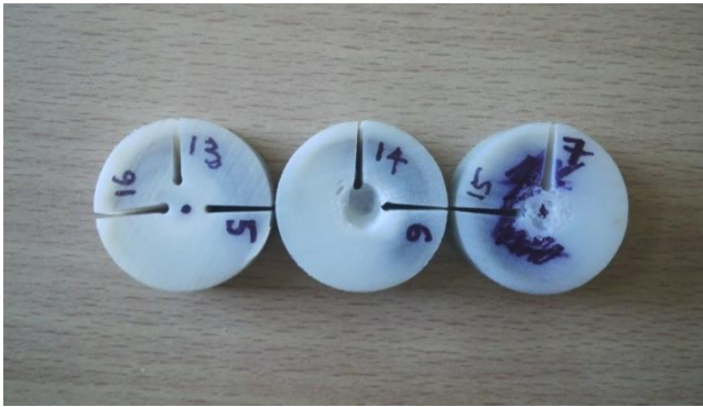
Fig. 2. Kerf angle of the machined surface
