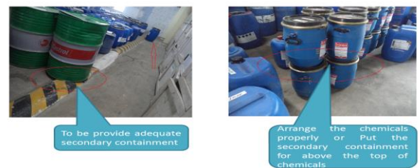
Fig 2 Improper Handling of chemicals using Tins
