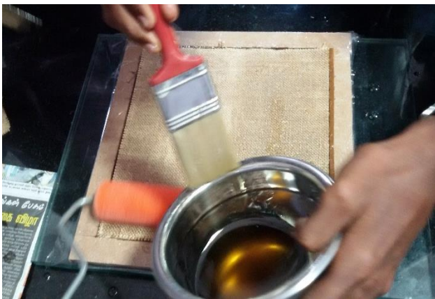
Fig. 2. Composite Fabrication by Hand layup technique
