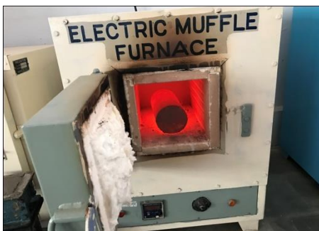
Fig 1. Cylinder in Muffle furnace
