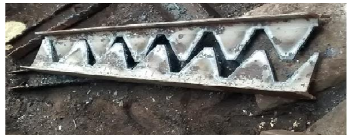
Fig. 2. Cutting of Castellated beam
