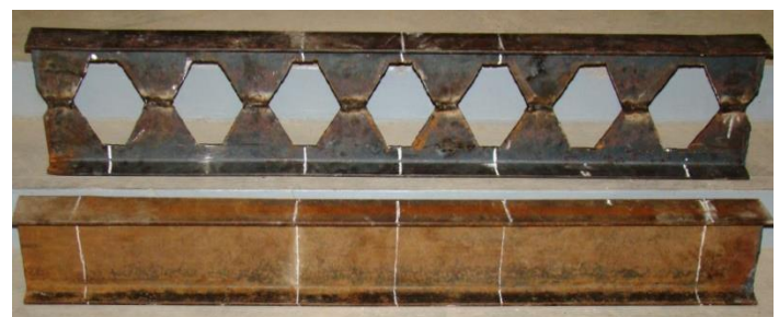
Fig. 3. Fabricated of Castellated beam
