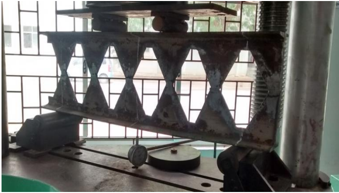
Fig. 4. Two point Load set up
