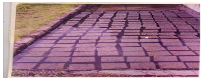
Fig.3. Curing of specimens
