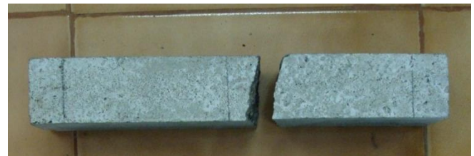
Fig. 10 Beam failure after testing
