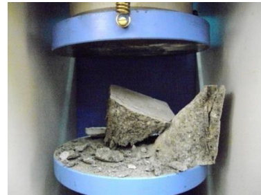
Fig. 4 Cube failure after testing
