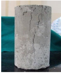
Fig. 6 Cylinder fails after testing
