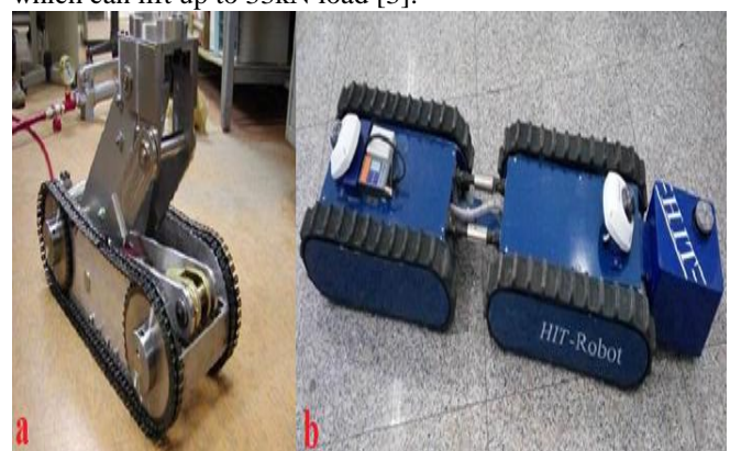
Fig.1. (a) Mobile Jack Robot for Rescue Operations [3]. (b) Multi-Link rescue robot [5].
